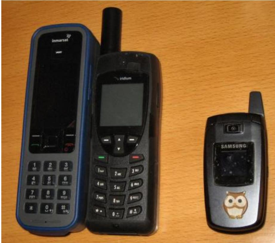
**Figure 1 Size Comparison of Inmarsat, Iridium, and Cellular Phone**
